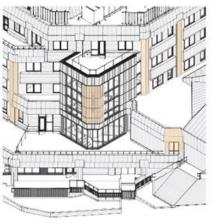
Proposed extensions to take precedent from existing chamfered detailing
